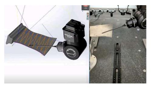
Revo auto programmed in CheckMate, simulation in SOLIDWORKS® on the left, Revo running the program on the right.
